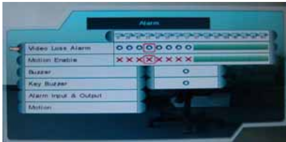
Figure 13.1 Alarm menu (8/16-channel)
